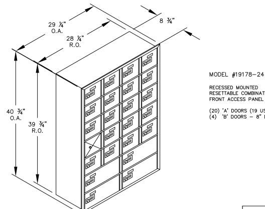
RESETTABLE COMBINATION LOCKS FRONT ACCESS PANEL (INCLUDES MASTER PANEL LOCK)
